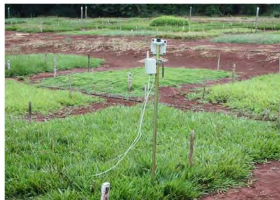
**Figure 2.** Wireless probes installed at two depths: 10 and 20 cm. To protect the transmitter it was enclosed in an IP68 protection code box.
